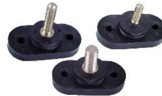
TST Studs Thermoplastic base with brass stud. Tested to 300 degrees and 400 amps continuous duty.
